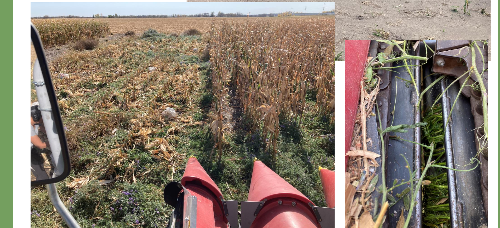
Harvest began Oct 6, 2021 and some issues with vetch growing upside of corn near the cob which wound around the stalk rollers. Recommend a high cobbing variety if going for grain.
